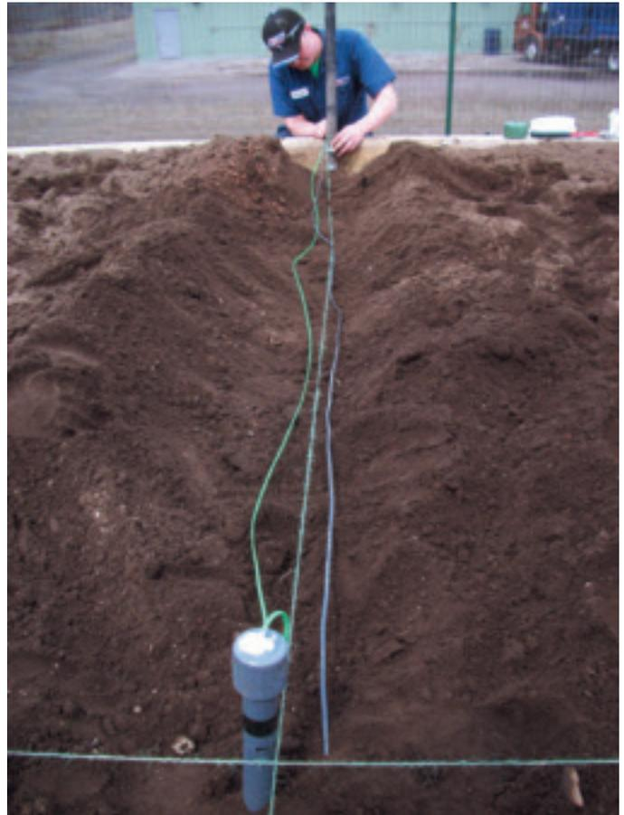
**SENSORS UNDER THE SOIL** — AGGRAND assistant Casey Lutz works to set up the line between the monitor and the moisture and temperature sensors that are implanted 12 inches below the surface in the growth plots.
